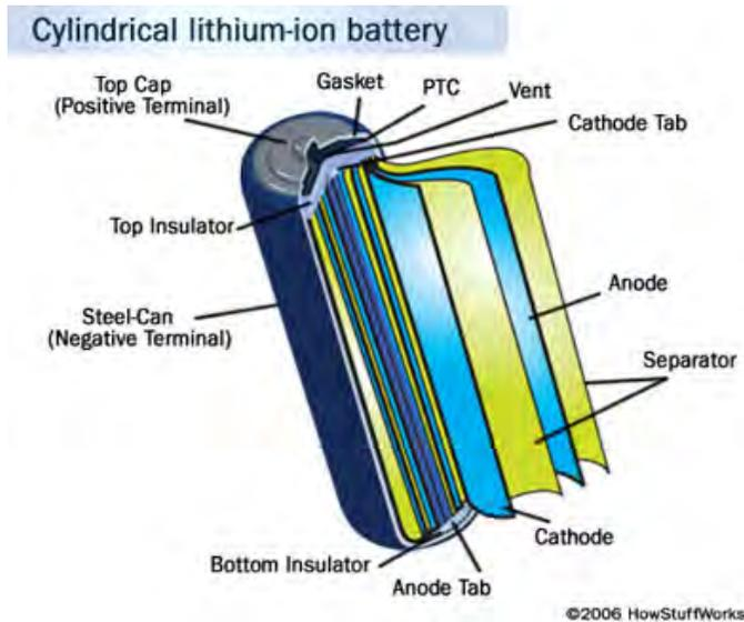
This metal case holds a long spiral comprising three thin sheets pressed together:
